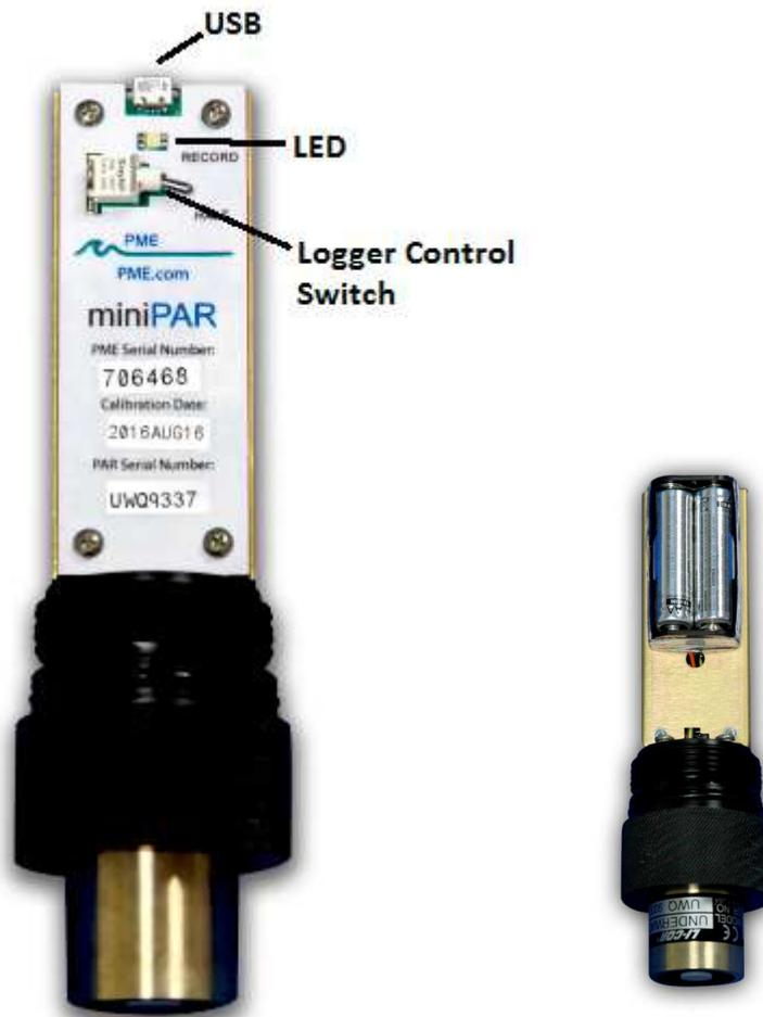
The **LED Light** is a LED that can display either red or green light. This is used to indicate the different features described in Chapter 1 in this manual.
