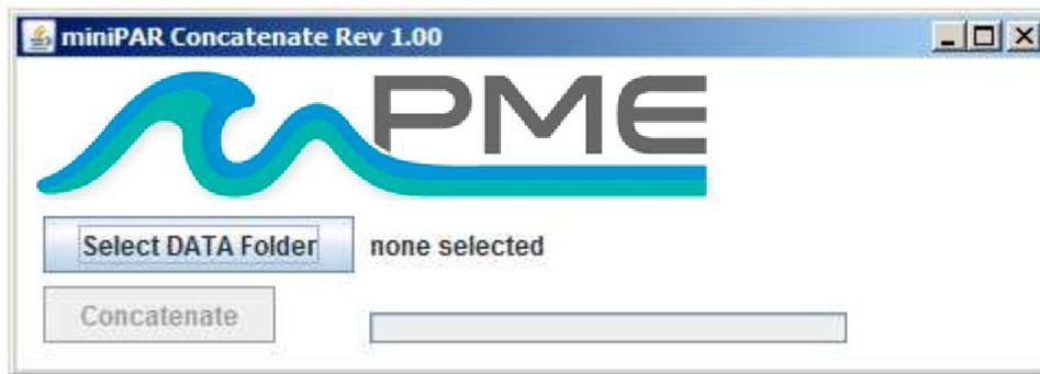
The miniPARConcatenate program reads and concatenates the files recorded by the miniPAR Logger. This program produces a CAT.txt file in the same folder as selected for the data. The CAT.txt file contains all the original measurements and contains two additional statements of time. CAT.txt is CSV (comma-separated values) file and can easily be imported into Excel and other database files.
