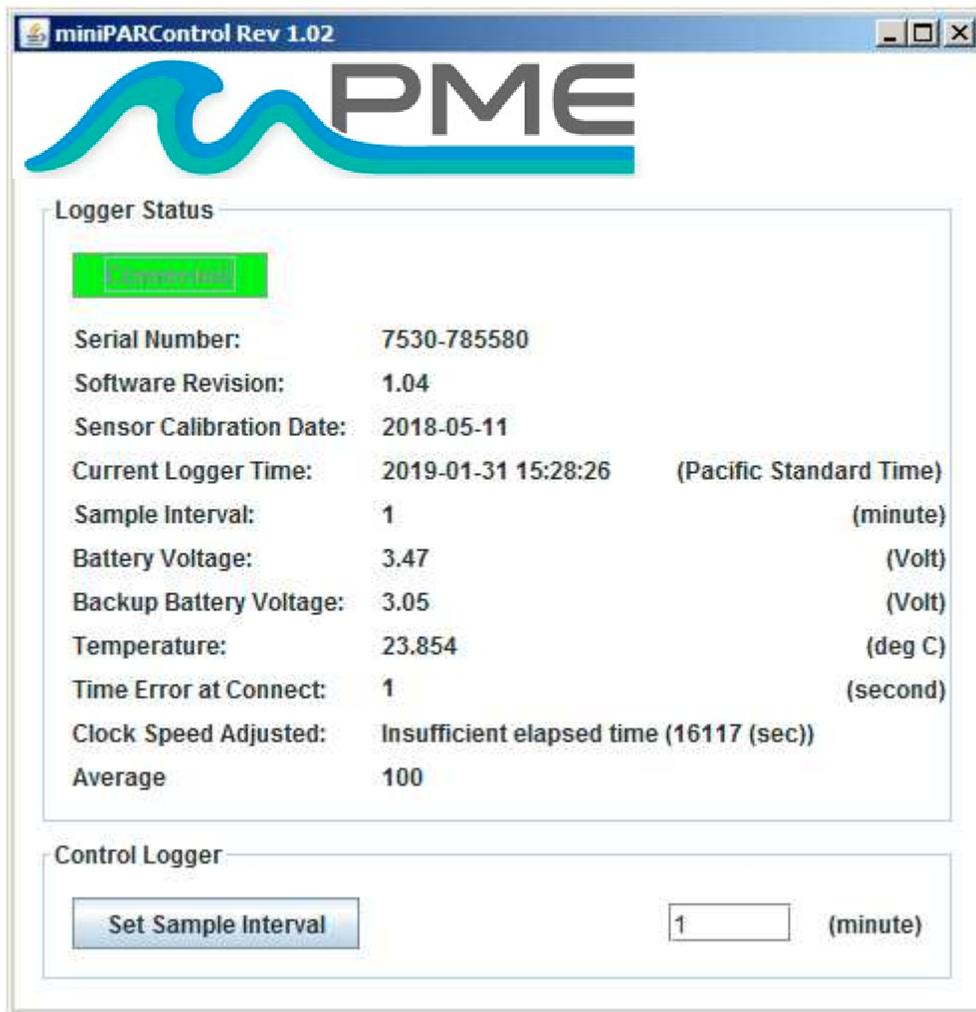
The miniPAR Logger must be connected to the HOST computer via the USB connection at this time. When correctly connected, the miniPAR Logger's LED will display a constant green light.
