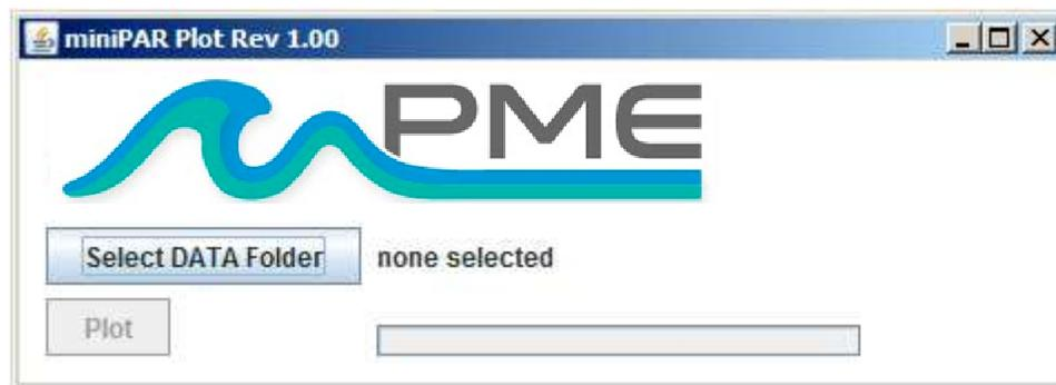
The miniPARPlot program plots the files recorded by the miniPAR Logger. The program reads all the miniPAR Logger files in a folder, except the CAT.txt file.
