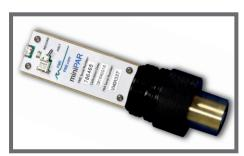
The miniPAR Logger is a completely submersible instrument that logs PAR (Photosynthetically Active Radiation), temperature and tilt measurements. The miniPAR sensor is a Li-Cor Underwater Quantum Sensor, https://www.licor.com/env/products/light/quantum\_underwater.html, which measures PAR from all angles in one hemisphere.
