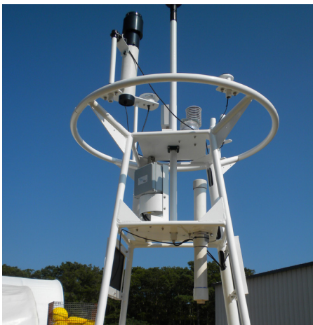
Figure 2. CO 2 -Pro Atmosphere Sensor measures both air and surface water pCO 2 for carbon flux measurements.
