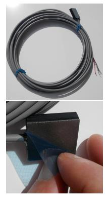
If the cable length of 25ft. is insufficient for the installation, additional cable can be added to the existing cable. If this is done, an accuracy-derating factor must be added to the overall temperature accuracy of this sensor. For every 100ft. of cable added, a derating factor of -0.125C must be taken into account.
