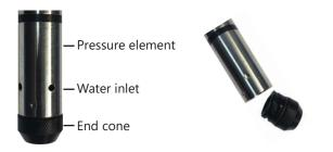
Gently twist off the end cone and carefully remove debris
