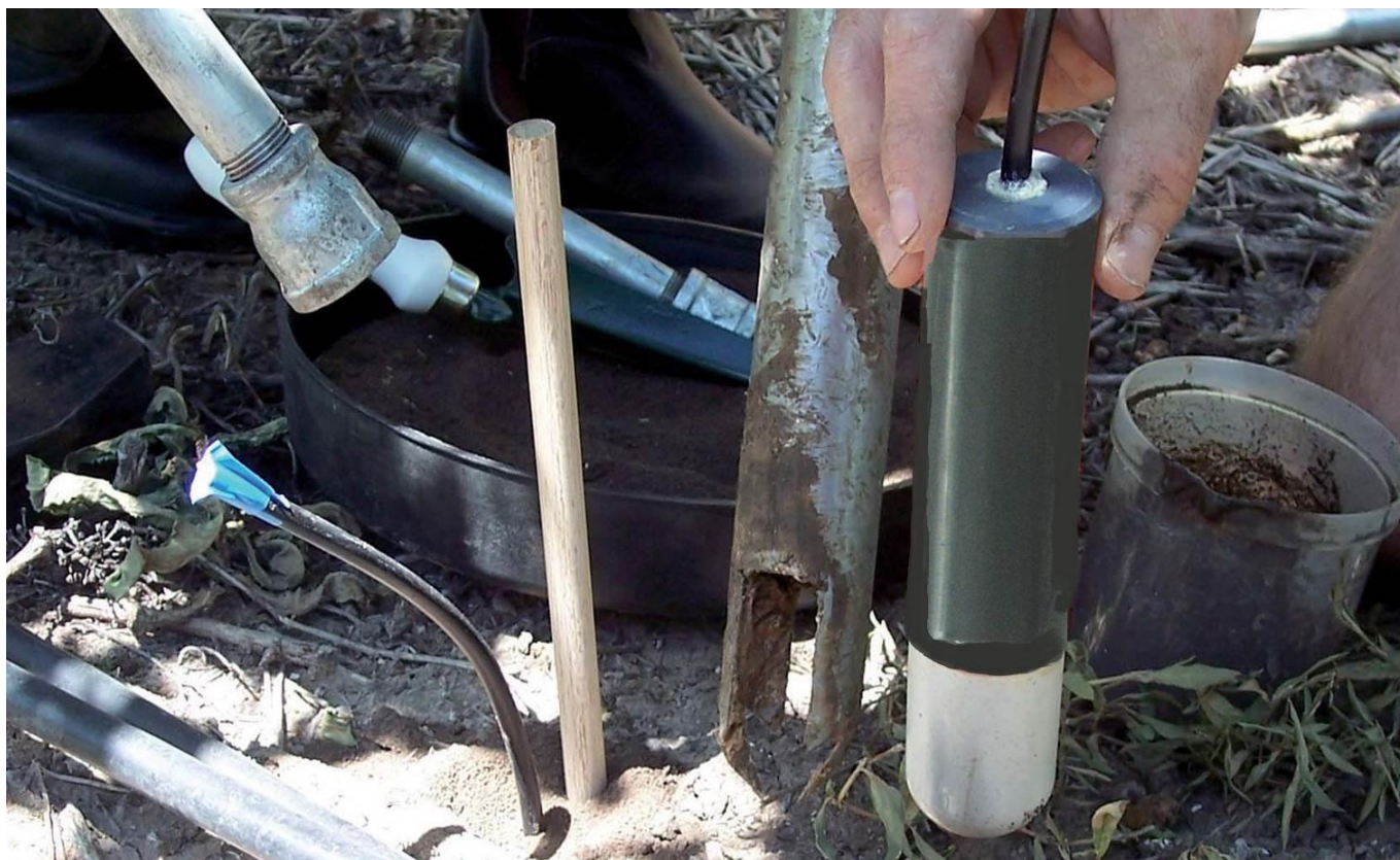
Figure 2. Equipment for installing the Sentek SoluSAMPLER™
