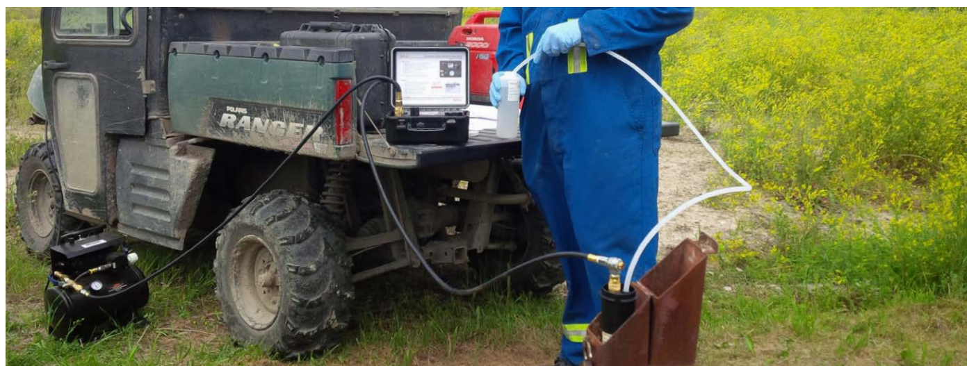
Groundwater Sampling with a Dedicated Bladder Pump using Portable, Rugged, Easy-to-use, Compressor and Controller
