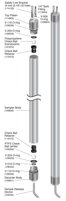
Model 425 1" dia. x 2 ft. Discrete Interval Sampler (114966)
