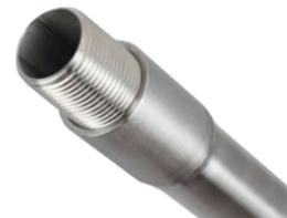
**1" NPTF to 3/4" NPTM Reducer Couplings** (113436) are available for installing a Levellogger in a section of 1" extension pipe. See separate installation instructions.
