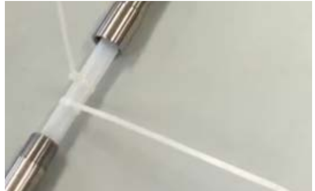
Cut and remove cable ties. Now slowly slide extension into place and tighten.
