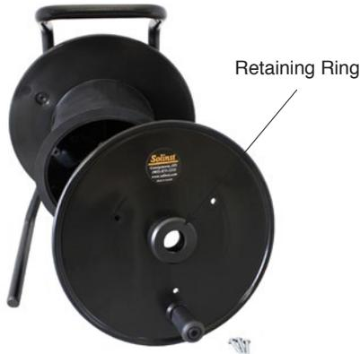
7. Feed the entire length of Direct Read Cable through the faceplate and reel hub until the Surface Connector seats in the retaining ring.
