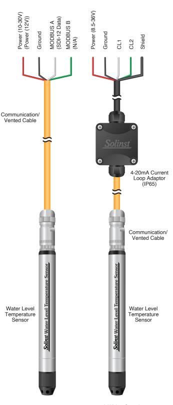
MODBUS Wiring Overview (SDI-12 in Brackets) 4-20mA Wiring Overview
