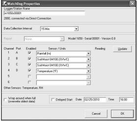
On the Properties screen, set the measurement interval, ranging from 1 to 60 minutes. The 1000 Series station has a capacity of 10,500 intervals, so it can record 209 days of data at a 30 minute interval.
