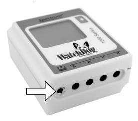
The **only time** you must have the WatchDog connected to the computer is during the launching and downloading of the data. After the station has been launched, and/or downloaded, disconnect the station and place it in the environment you wish to monitor.
