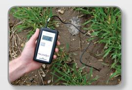
FieldScout Soil Sensor Reader connected to a buried WaterScout SM 100 Soil Moisture Sensor.
