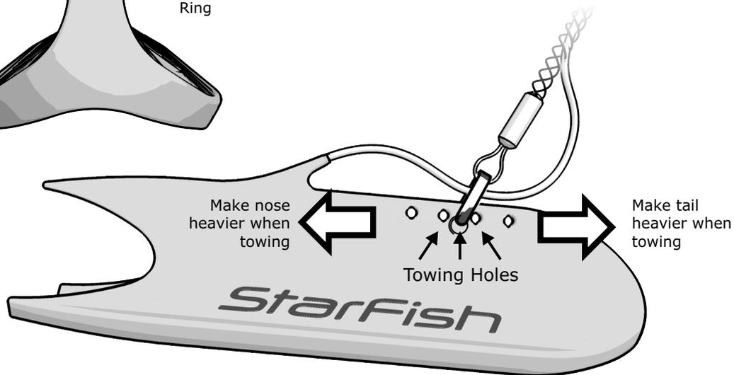
Depending on the salinity of the water and the towing speed of the sonar you may find that you need to adjust the towing position backwards from the middle towing hole to achieve the best results. However, only the three central holes are intended as towing points (the outer holes are for use in transit and the attachment of accessories).
