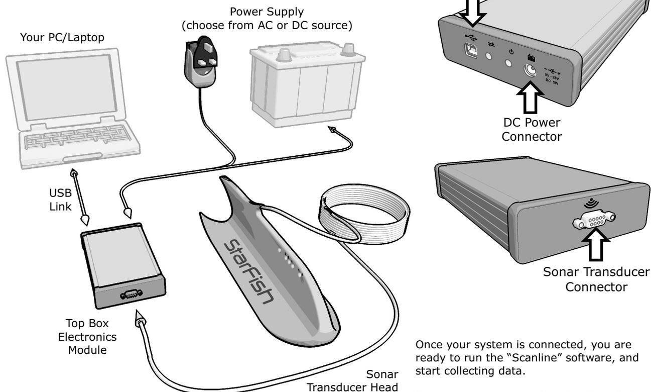
Once your system is connected, you are ready to run the "Scanline" software, and start collecting data.
