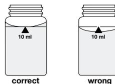
● **Avoiding errors in photometric measurements**
