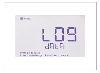
Critical data is automatically saved to the meter's 500-point data log.
