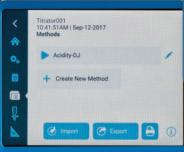
Customizable methods save electrode, titrant and sample titration settings so routine procedures can be repeated without additional setup or pre-work and methods can be shared among titrators using a USB flash drive.
