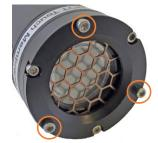
CAUTION: It is important to ensure the copper screen does not contact the stainless steel head cap screws or the sensor membrane as this will result in galvanic corrosion of the head screws. If the Pumped Head Assembly is used the copper screen can be used but you must install longer screw
