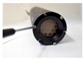
CAUTION: Be careful not to damage the membrane, the hex driver can easily puncture the membrane if it slips. It is recommended to alternate sides when removing the screws to release the faceplate evenly.
