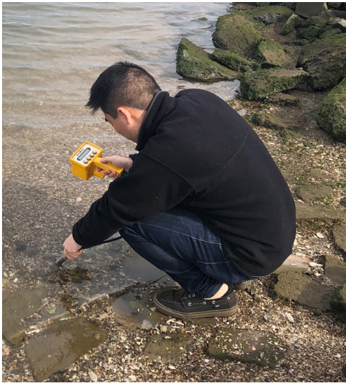
Configure Analog Probes with DataBank Handheld Datalogger for field sampling
