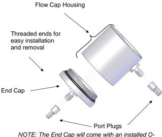
NOTE: The End Cap will come with an installed O Ring that should not be removed for sealing purposes.
