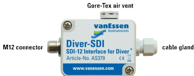
Figure 1 top view of the Diver-SDI (part no. AS379).
