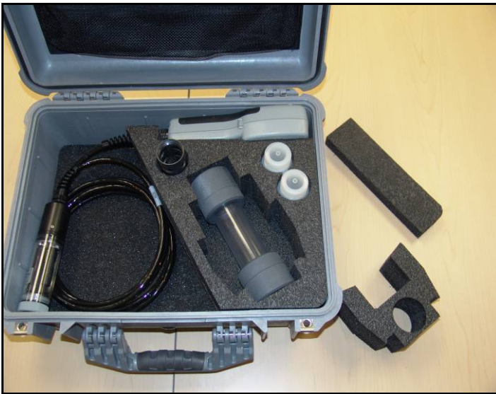
3074 case shown with 556 instrument and 3059 flow cell. Instrument spacer and flow cell spacer removed. The cable is connected to the instrument.
