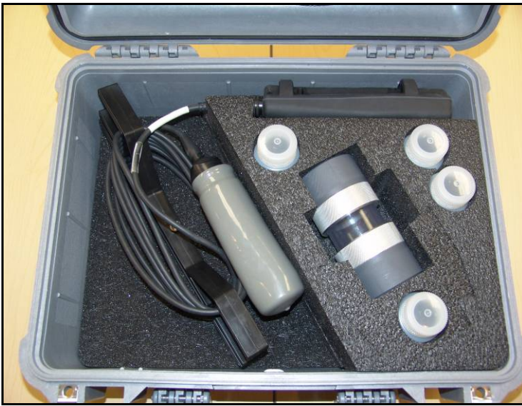
3074 case shown with Pro Plus instrument and 6850 flow cell. Instrument spacer and flow cell spacer installed. The cable is connected to the instrument and is wrapped on a 3062 Cable Management Kit.
