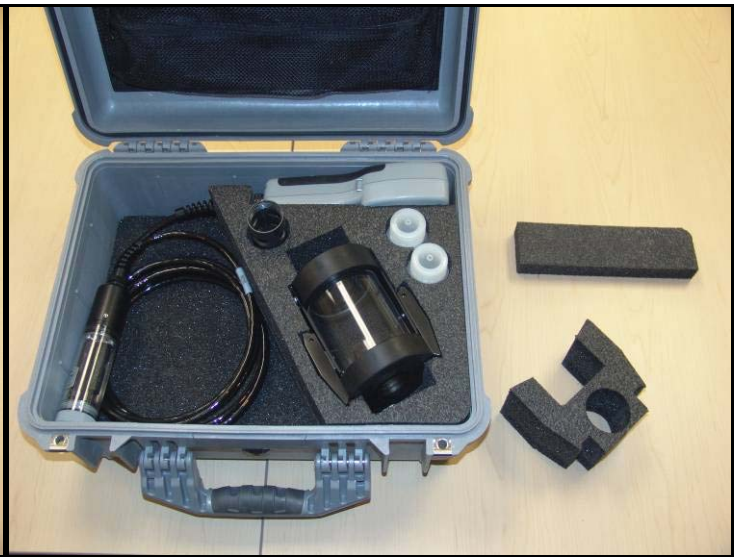
3074 case shown with 556 instrument and 5083 flow cell. Instrument spacer and flow cell spacer removed. The cable is connected to the instrument.
