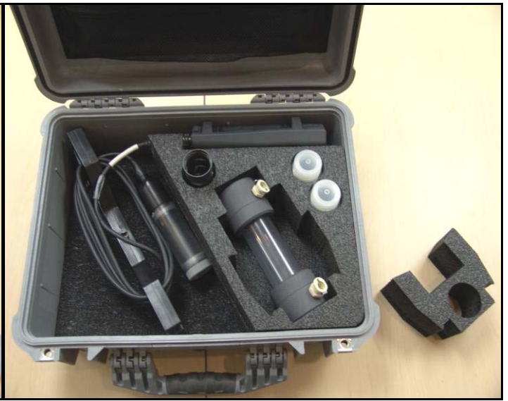
3074 case shown with Pro Plus instrument and 3059 flow cell. Instrument spacer installed and flow cell spacer removed. The cable is connected to the instrument and is wrapped on a 3062 Cable Management Kit.
