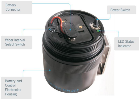
FIGURE 6: INSIDE THE HYDRO-WIPER A CONTROL HOUSING
